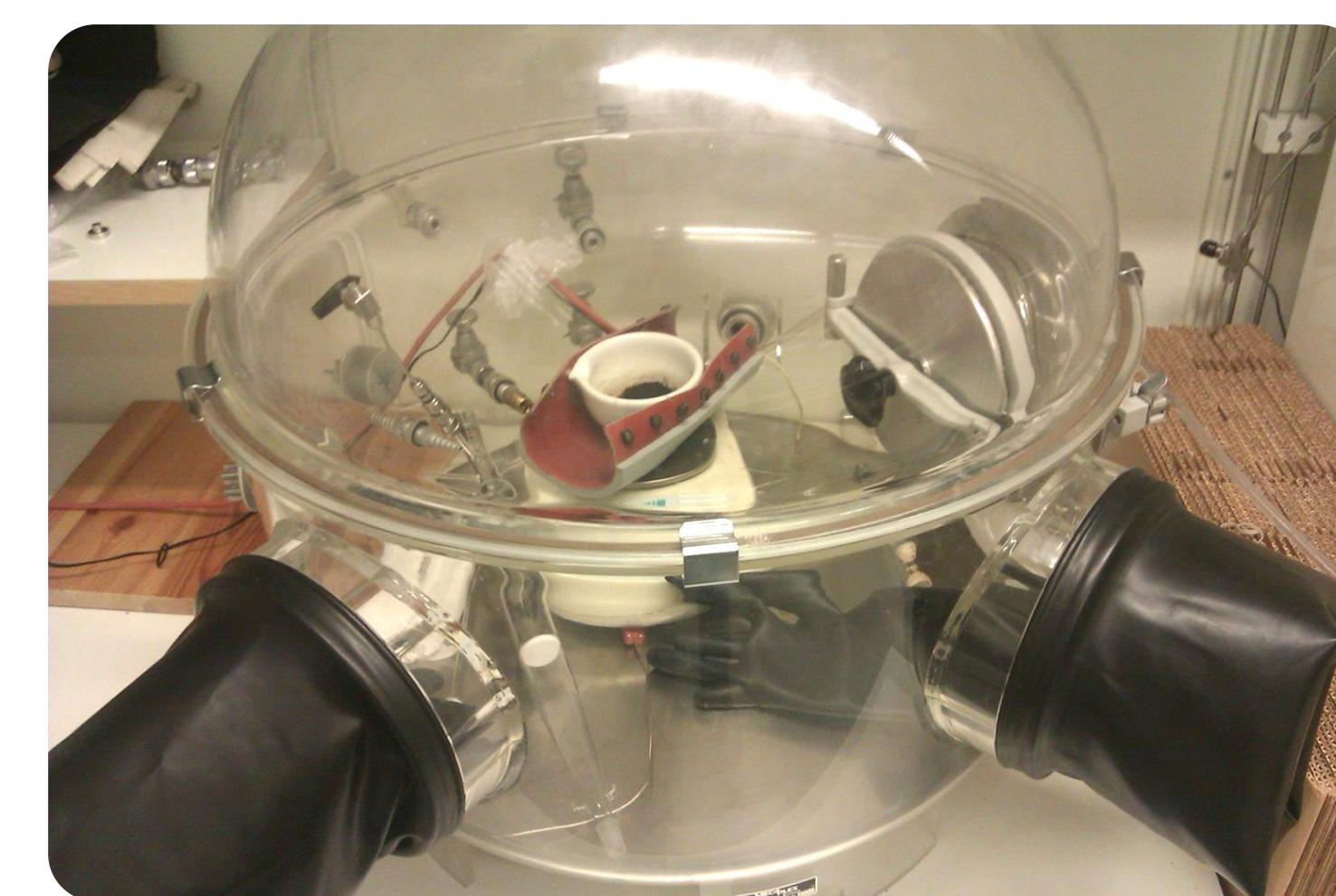
Chamber used for sulphur addition in inert atmosphere
